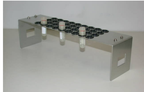
Figure 1: 1.5 (2) mL tube rack TR-4002 (Micro tube mixer MT-400 supplied rack; TOMY Digital Biology Co., Ltd.)
